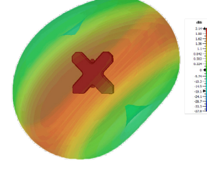
3D Pattern Element 2 (2100MHz)
